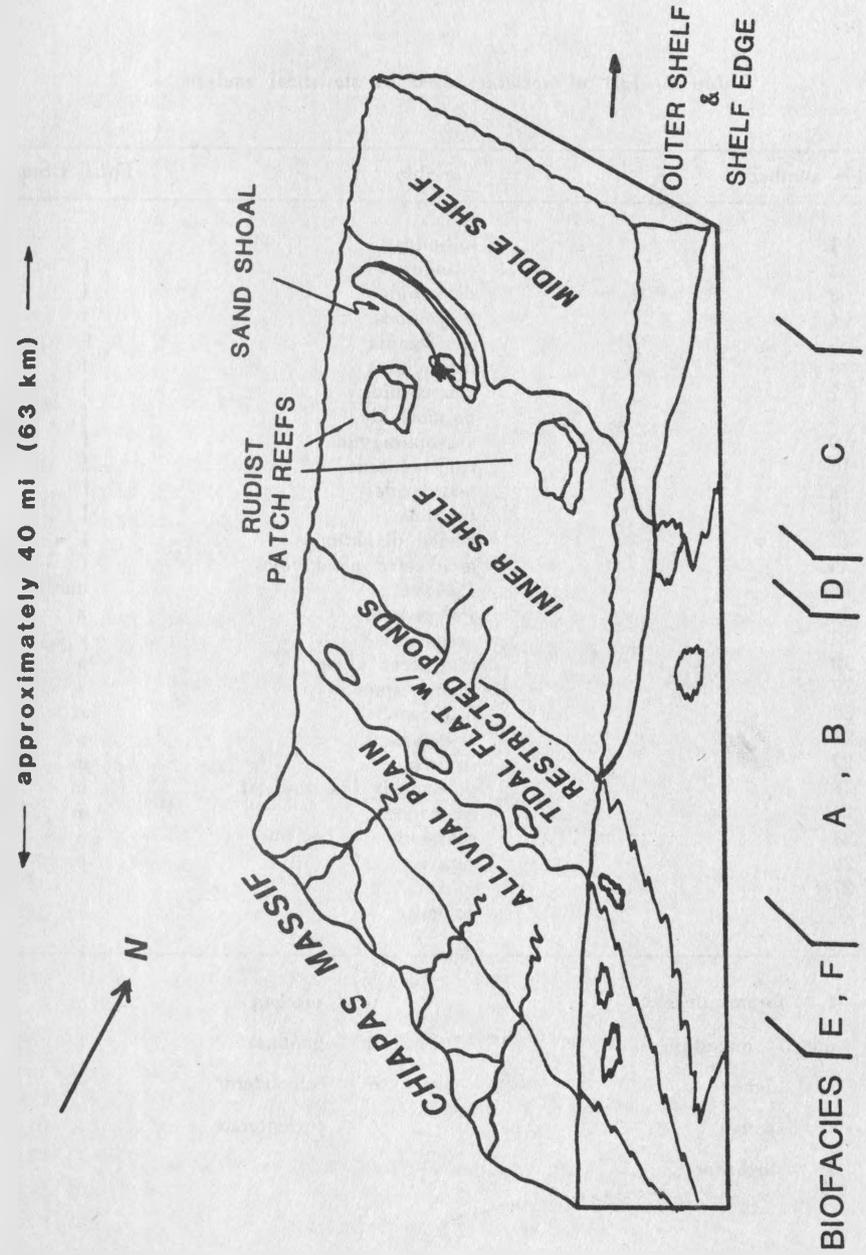
FIGURE 19.—Depositional model for the Sierra Madre Limestone in west-central Chiapas.
