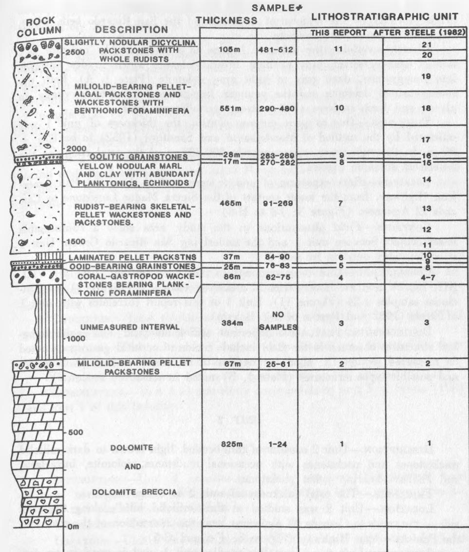
FIGURE 11.—Generalized rock column and lithologic units of the Sierra Madre Limestone, west-central Chiapas.
